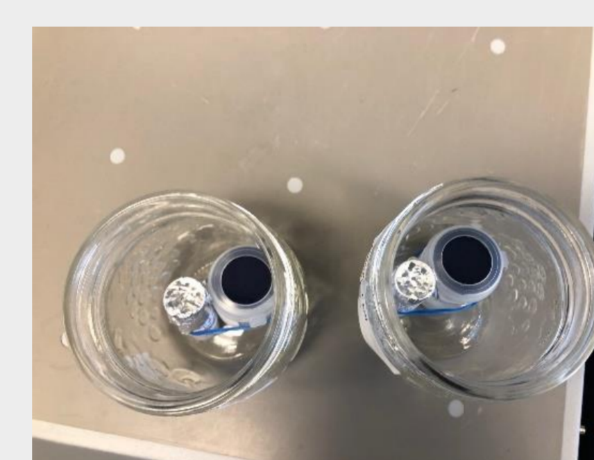
Representative ASAP sample with saturated salt solution in vial with Gore-Tex lid, and sample with perforated foil covering.
